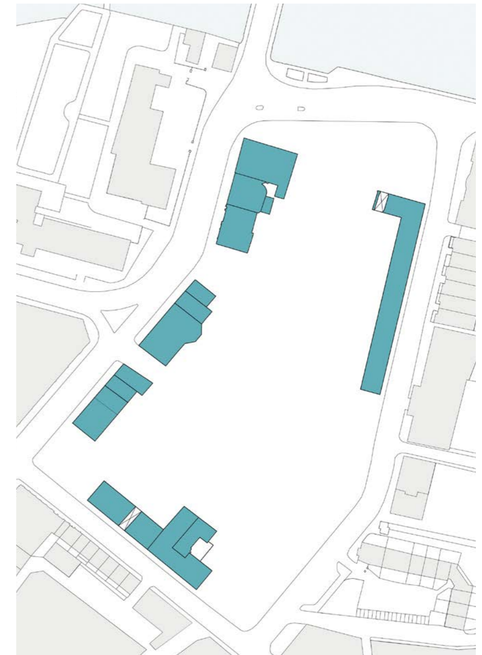
Fig. 18: The buildings to be retained will require varying levels of refurbishment depending on their condition, layout and proposed use
